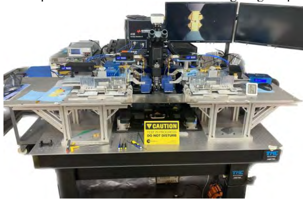
Figure 2. D band fully calibrated vector LP setup with external downconvertors
